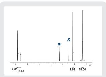
Figure 2. <sup>1</sup>H-NMR spectrum of 5.3 mg of 2,6-di-tert-butyl-4methylphenol in DMSO-d<sub>6</sub> with 100 ppm D<sub>2</sub>O added. Note the reduced ratio of the phenolic proton 18:3:2:0.47 (t-butyl: methyl: ring-H: -OH). Note that the HOH and HOD peaks are separated in the spectrum.
