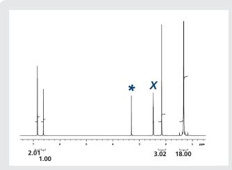
Figure 1. 1H-NMR spectrum of 5.0 mg 2,6-di-tert-butyl-4-methylphenol (MW 220.36g/mole) in dry DMSO-d<sub>s</sub>. Note the proper integral ratios of 18:3:1:2 (t-butyl: methyl: ring-H: -OH). Note the single H<sub>2</sub>O peak at 3.3 ppm.
